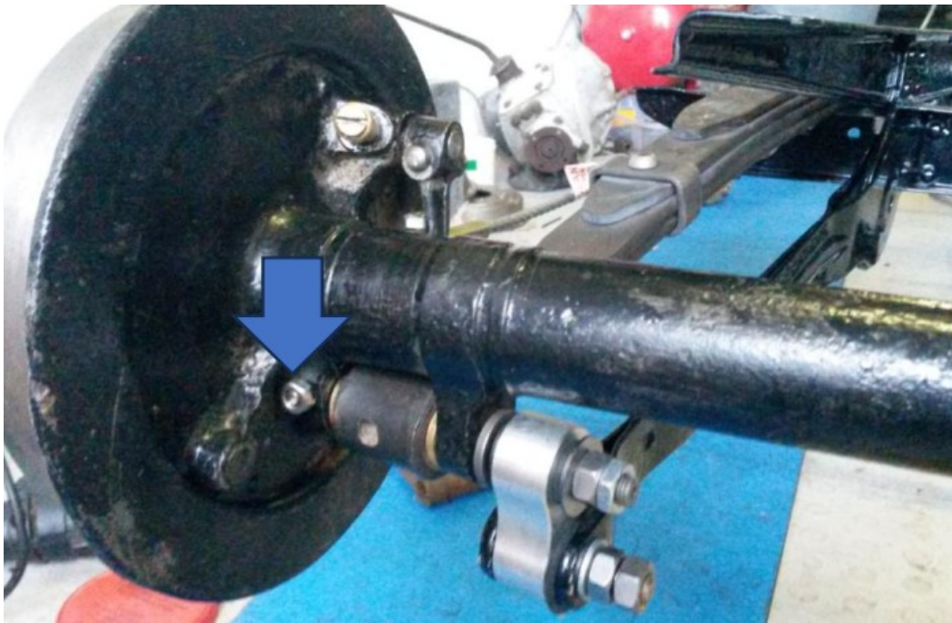
Rear axle casing with spring attached, and shock absorber attached via shackle to spring pin. Note nut of cotter pin (blue arrow)
