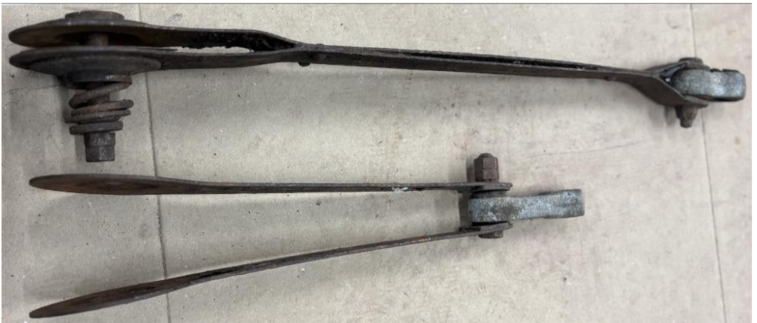
The rear damper on a Ruby (bottom) is shorter than on the earlier Box saloon (top)
